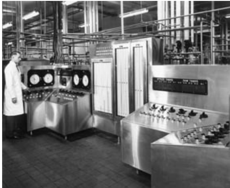
The controls to pasteurization, distribution and packaging machines. Dairyland plant in Burnaby, B.C. 1964. Source: Dairy Industry Society of BC
